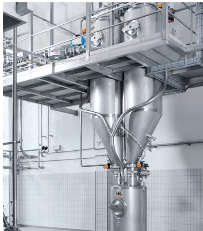
Two asymmetric receiver with butterfly valves for discontinuous conveying
