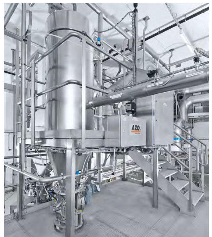
Receiver with rotary valves for continuous product conveying
