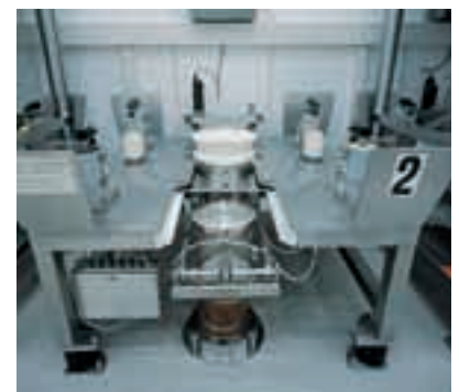
Docking station for interchangeable containers with metering screw
