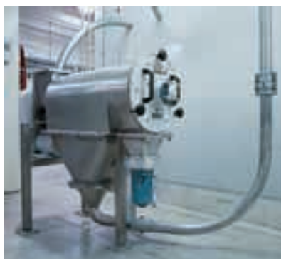
The in-line Cyclone Screener becomes an integral part of the conveying system
