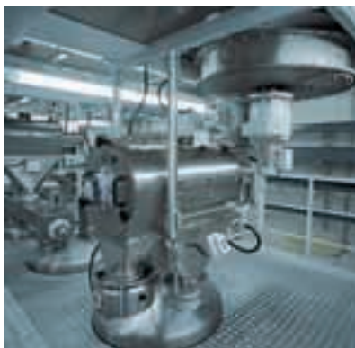
The in-line Cyclone Screener becomes an integral part of the conveying system
