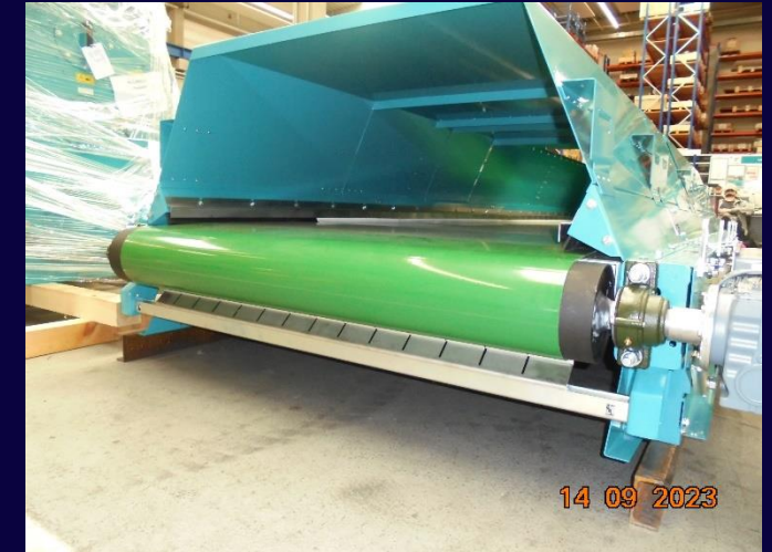
Green belt is antistatic ⇒ For non Atex machines only)
