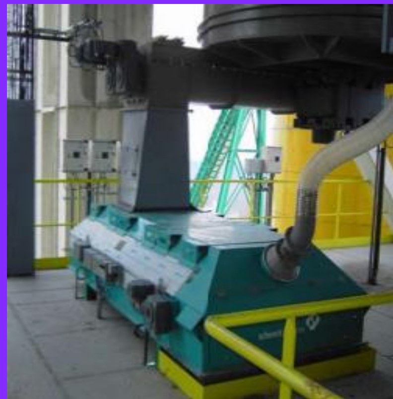
MTD-E incl. Pre-bin with extraction screw and piping to the filter “AF version - sealing around the infeed”
