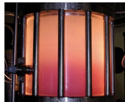
The wash column with visible wash front
