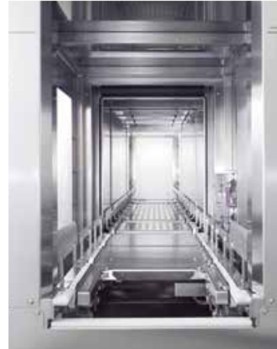
Inline system with circulating air heating zones and a vacuum drying zone.
