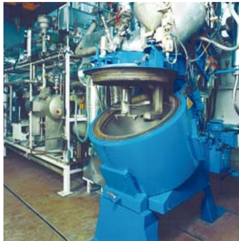
Fig.14.2: Mixing reactor Type R08VAC in the pilot plant, shown with the cover and mixing tools raised
